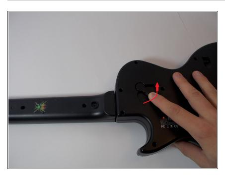
Pull the Lock on the back of the body to detach the neck from the body.
