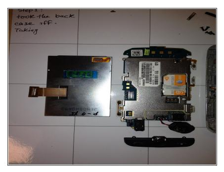
Separate the display plate from the circuit board by pulling on the orange wire tape that connects the black rectangle at the edge of the wire tape to the circuit board.
