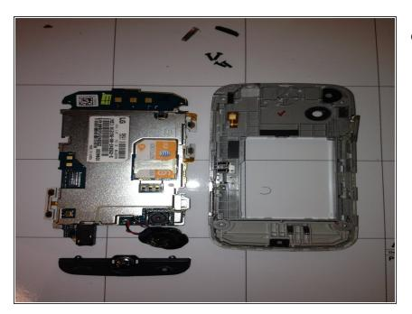
Use a pair of thin tweezers to carefully pry the rectangular display plate from the front casing. Slide one of the sharp ends of the tweezers between the display plate and the plastic case and lightly apply pressure until the plate pops out. The display plate will still be attached to the circuit board by a single strip of orange wire tape.
