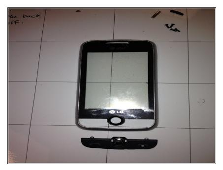
At this point, you should be able to easily pull off the small console at the base of the phone, below the screen, that contains the circular silver home button.
