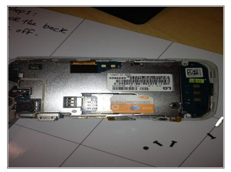
Next, extract the orange and white plastic SIM card from the back of the phone by using a finger to slide it out from underneath the thin metal bar that holds it in place.
