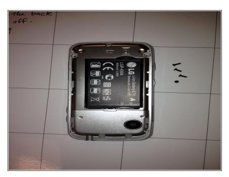
Remove the plastic shell that covers the back of the phone by applying pressure with two fingers in a downward sliding motion.
