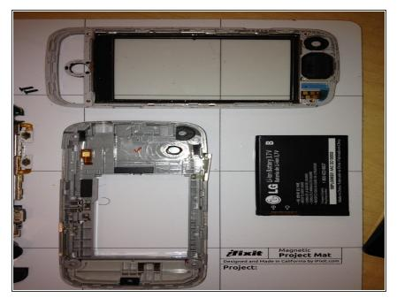
Remove the black, rectangular battery labeled LG Li-Ion Battery (3.7V) by lightly applying pressure to the center. The battery should pop out.
