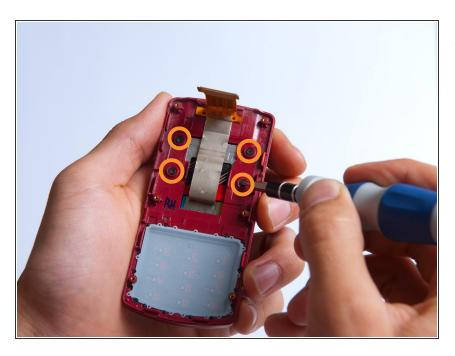
Take the front case and unscrew the four Phillips #000 (1mm) screws around the ribbon.
