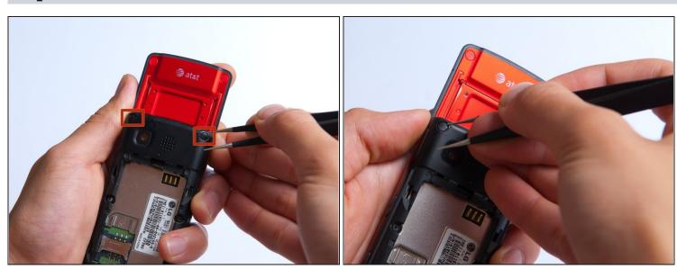
Remove the two screw covers at the top of phone with tweezers.
