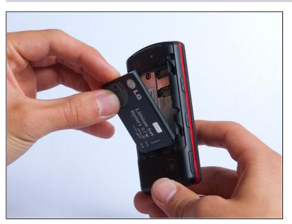
• Lift and remove the battery.
