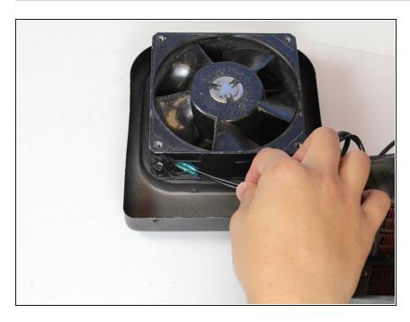
Unplug the two blue wires that connect the fan to the Power/Fan Switch Circuit Board Assembly by pulling them away them from the fan.
