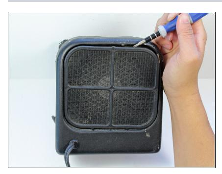
Gently pry the back screen off of the device using a flathead screwdriver and remove it.
