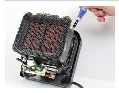
Remove the 10 mm screw that attaches the fan to the heating coil assembly using the #2 Phillip Screwdriver.
