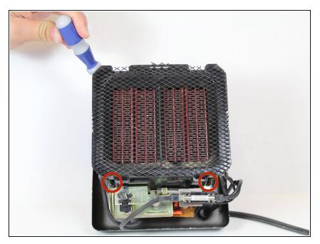
Remove the three 10 mm screws that attach the fan to the heating coil assembly using the #2 Phillip Screwdriver.
