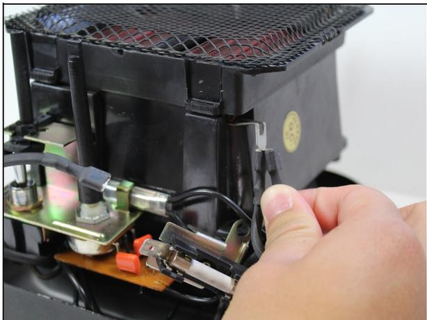
**i** Make note of where you disconnect the wires from so you can properly connect them when re-assembling heater.
