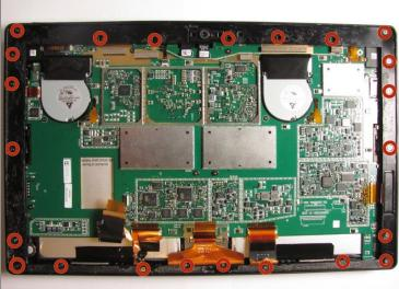
• Using a T5 Torx screwdriver, unscrew a total number of 23 screws located on the outside panel of the Surface Pro.
