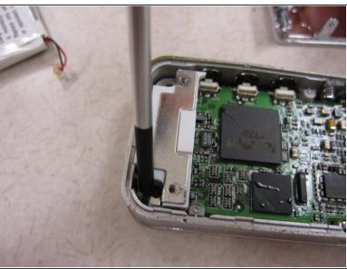
Using the philips screwdriver, remove the two screws on the mother board.
