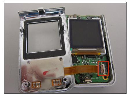
After opening the front cover you will see and electric ribbon connecting the buttons to the mother board.
