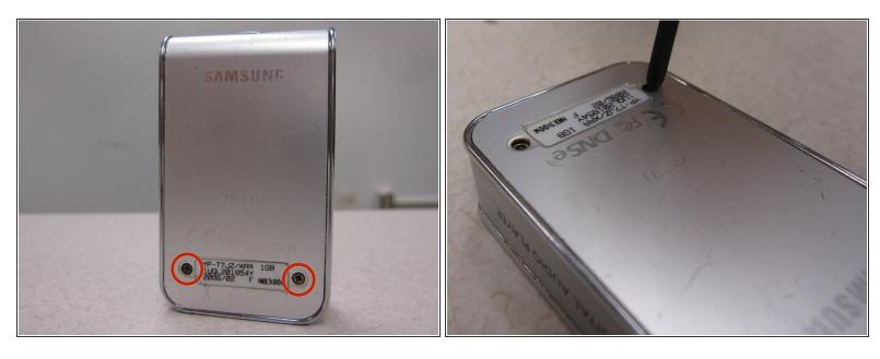
Remove the 2 screws on the back cover using a Phillips head #0 screwdriver.
