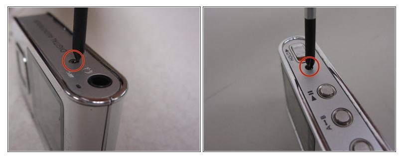
• Remove the screw on each side of the device using a Phillips head screwdriver.
