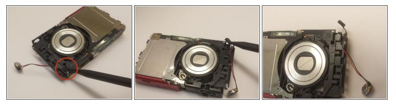
• With the camera laying with the lens up, use the spudger tool to grab the small square piece of rubber and gently pull it out.
