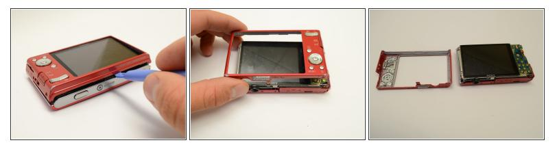
• Flip the camera over 180 degrees and similarly pry off the rear casing.
