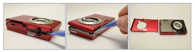
• Use a plastic opening tool to carefully pry off the front casing.
