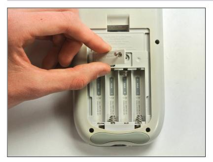
Grab the plate and lift gently upward, to remove the backup battery cover.
