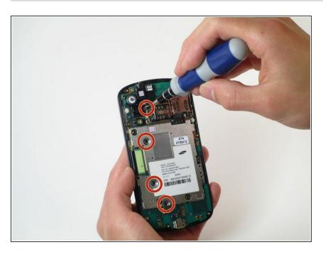
Remove the four black 3mm screws securing the motherboard with the Phillips #000 screwdriver.
