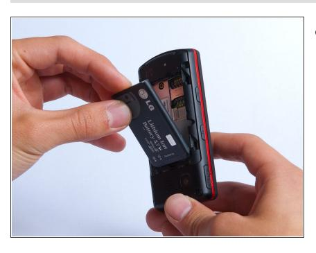
Lift and remove the battery.
