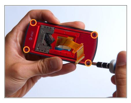
Unscrew the four Phillips #000 (3mm) screws at the corners of the phone.
