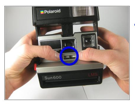
Locate the exposure setting switch under the main lens on the face of the camera.
