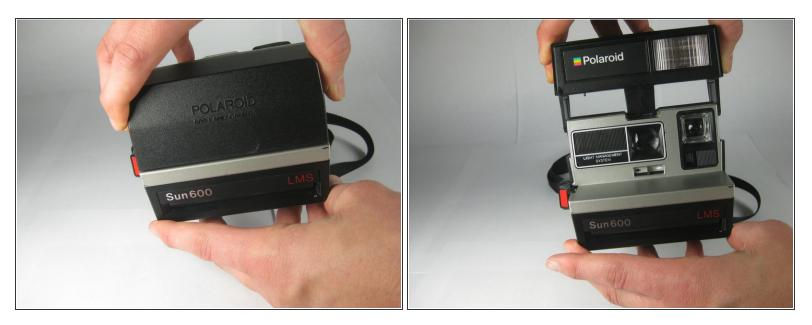
• Open the flash assembly by holding the sides of the top piece of the camera and pushing up gently until it snaps into place.
