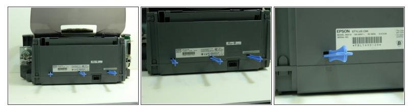
• Turn the printer around so the front is facing away. Use three wide-tip blue plastic opening tools and place them inside the notches on the back panel of the printer.
