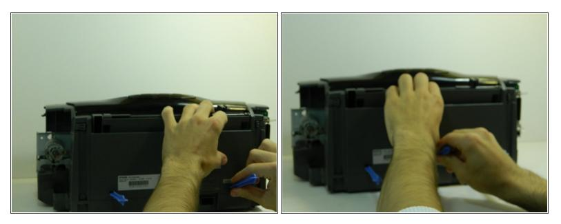
• Push on each notch until the retaining tabs are separated from the back plastic cover.
