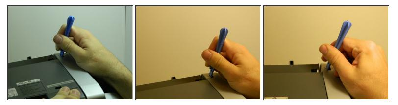
Wedge a wide-tipped blue plastic opening tool inside the gray tab on the upper left-hand corner of the right panel, next to the arrow.
