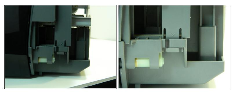
• Turn the printer around so the front is facing you and gently push up on each tab of the front plastic panel, above the arrows. Make sure the prongs are detached from the clips.
