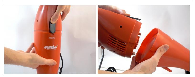
Press the black separator switch and lightly pull the bottom half away from the top.
