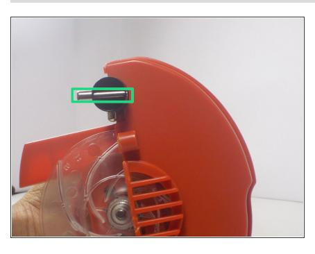
Once the housing is open, locate the solid chrome plated piece at the front end of the extendable pole.
