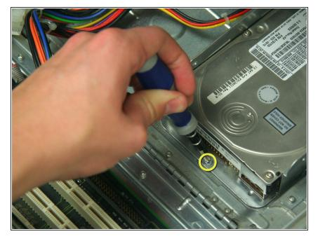
Remove the screw which holds the Hard Drive tray in place.
