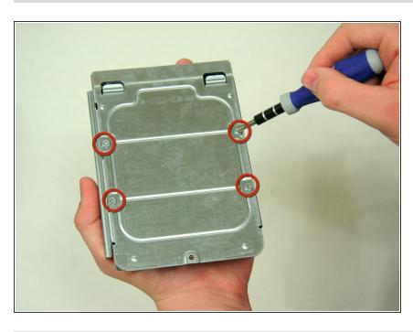
To remove the Hard Drive from the tray, unscrew the 4 screws on the bottom of the tray.
