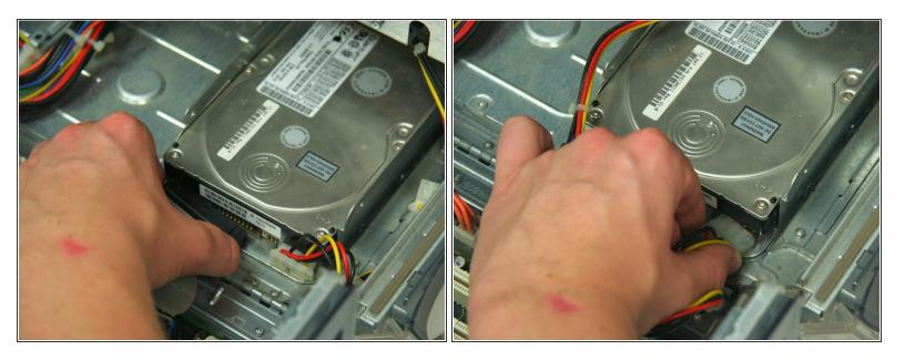
Remove the ribbon cable and power cable from the Hard Drive.
