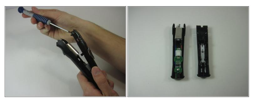
• Pry open the plastic cover into two separate pieces. The plastic is very durable so don't worry about breaking it upon prying it open.
