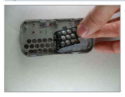
• Once the circuit board has been removed the rubber keypad will be visible. If it has not fallen out on its own it can simply be peeled out. It is lightly attached like a sticker on the top three tabs. The left most table is labeled "B", the center tab is blank, and the right tab is labeled "N".
