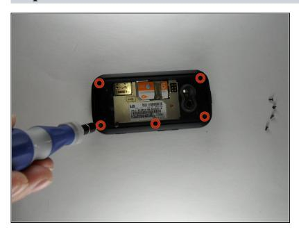
Remove 5 screws, 1 from each corner of the phone and 1 from the center-right of the phone.
