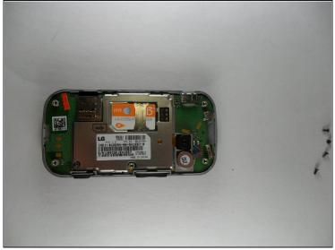
Now pull off the rear casing, using an opening tool. \*\*Buttons for volume and pictures may fall out\*\*
