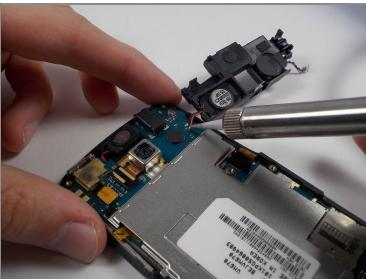
Use a soldering iron to desolder the connections attaching the the antenna to the motherboard.
