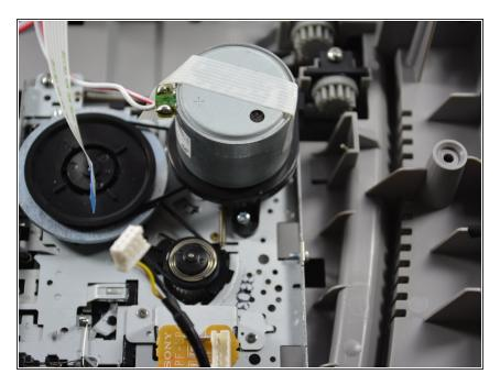
• Push the motor back down and screw it into place.
