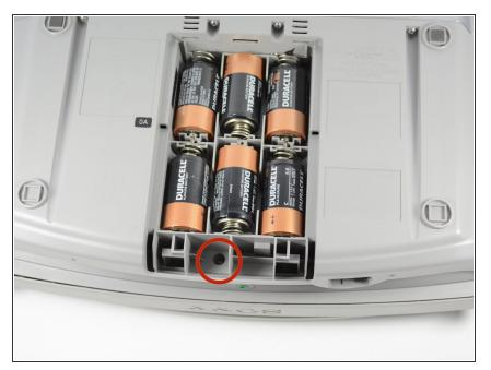
• Flip the radio upside down and remove the battery cover. Unscrew the one screw below the batteries.
