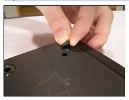
Pop off the front two rubber footings from the bottom of the device, revealing 2 hidden main panel screws.
