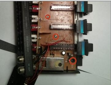
Remove all six screws from the circuit board.
