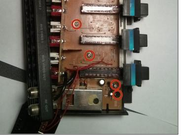
• Correctly place the circuit board back into the case of the device and replace all six screws on the circuit board.
