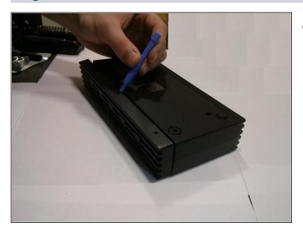
Carefully pry off the front panel of the device.
