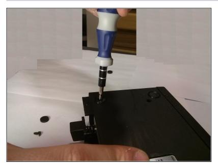
Unscrew the remaining 7 screws from the bottom of the device.
