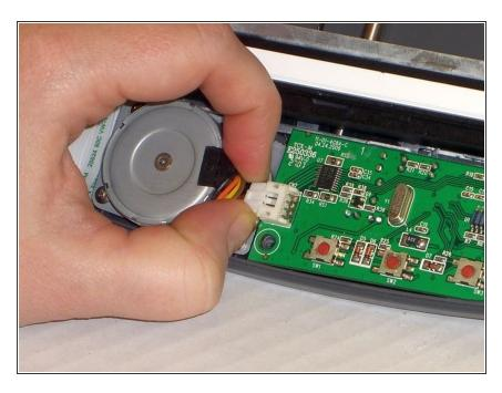
Carefully detach the wires from the motherboard, pulling slowly but firmly.
