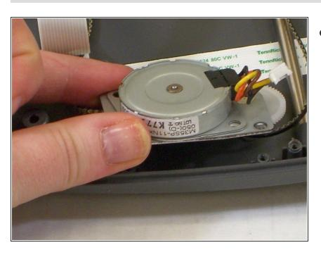
Lift the motor out of the scanner.
