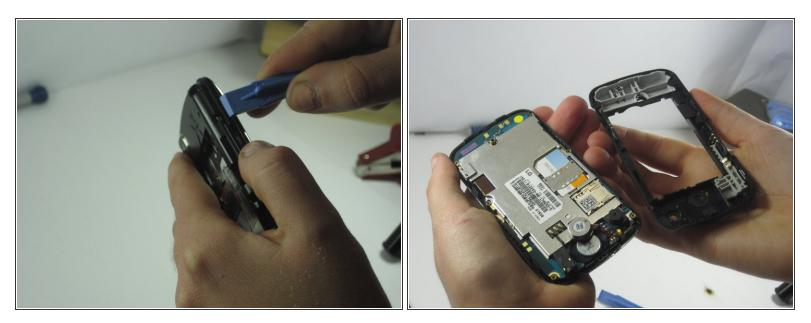
• Place the opening tool in the seam of the device and pry around the perimeter to separate the top case from the bottom case.
