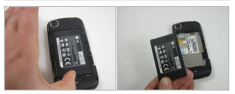
• Use your fingers or a spudger to remove the battery. Lift it from the side opposite of the camera.
