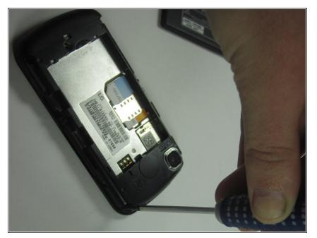
Use a Phillips #0 screwdriver to remove six screws around the perimeter of the phone.
