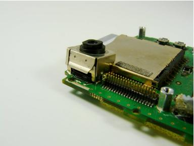
• Using the flat end of the spudger, lift the metal case off of the camera.
