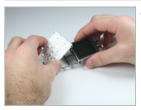
Lift the keyboard out of the plastic frame.
