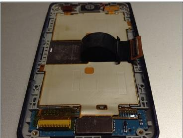
• Remove the slider plate. This can be done by inserting a plastic card or thin pry tool between the colored top plate and the slider plate. Once inserted carefully work the card around the edges until slider plate pops off. **Note:** This can be tough to open the first time
