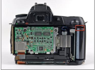
• Pull the rear cover off the body of the D70, minding the LCD board ribbon cable that may get caught.
