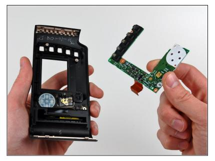
Remove the LCD board from the rear cover.
