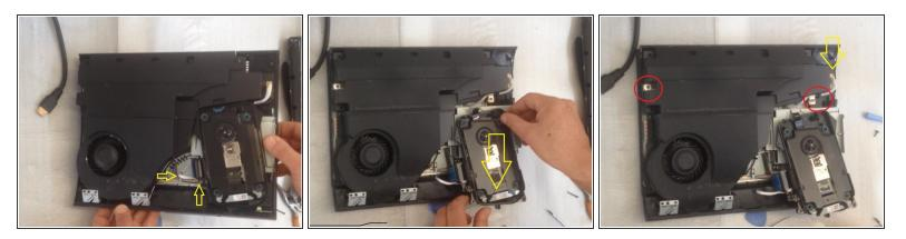
• Disconnect two flex-cables and move the Laser Unit. Remove the two screws and the small cable and then take out the Power Supply Unit.
