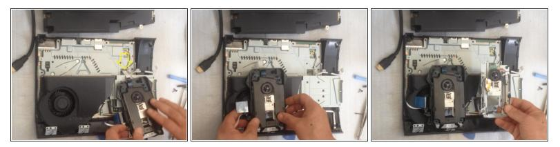
• To release the laser unit disconnect this flex-cable.
