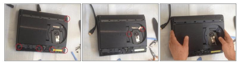
• Remove 7 screws to release top cover.
