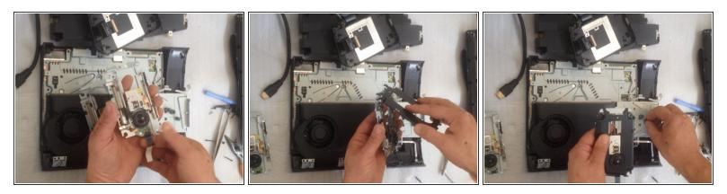
• Disconnect this flex-cable and attach it to the new spare part. Let's start assembling.
