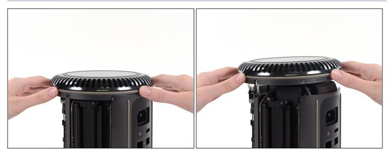
• Carefully lift the lower case up and remove it from the Mac Pro.
