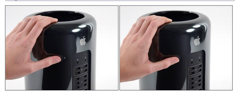
• Slide the lock switch to the right, to the unlocked position.
