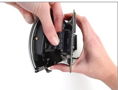
Squeeze and pull the audio jack ribbon cable connector from the IO board.
