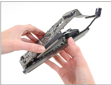
Lift the IO board up from the IO shield from the end with the AC plug.
