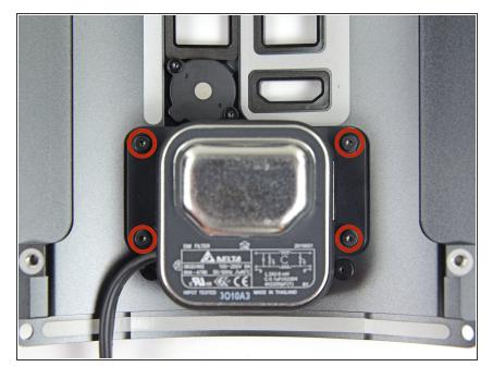
Remove the four 6.5 mm T4 screws (with washers) from the flange around the AC socket.
