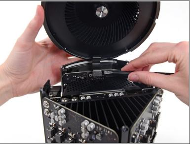
Use the flat end of a spudger to disconnect the fan assembly ribbon cable from the IO board.
