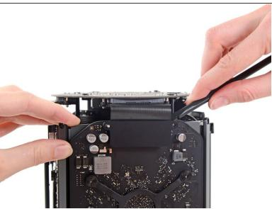
Use the flat end of a spudger and a twisting motion to gently separate one side of the graphics card data connection.
