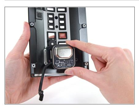
Remove the AC socket from the IO panel.
