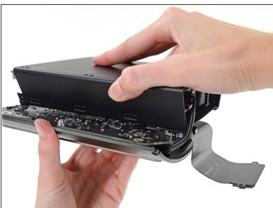
Gently shift the power supply to free the AC power inlet cable out of its plastic clip.
