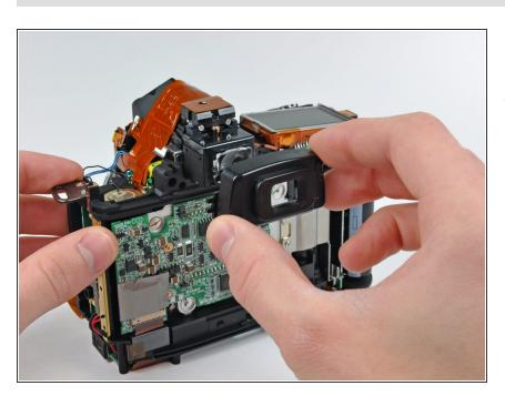
Carefully remove the eyepiece from the D70. To reassemble your device, follow these instructions in reverse order.
