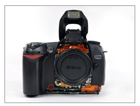
Remove the 4.2 mm Phillips screw securing the lower edge of the grip to the front of the D70.
