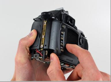
• Carefully pull the sides of the rear cover away from the body of the D70.
