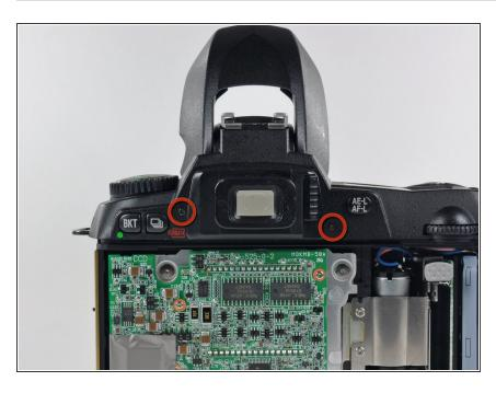
Remove the two 7.3 mm Phillips screws securing the top case to the D70 near the eyepiece.
