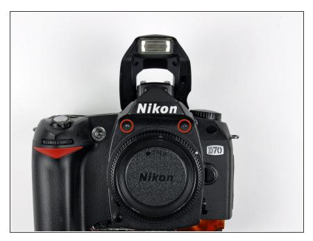
Remove the two 4.3 mm Phillips screws on the face of the front cover.
