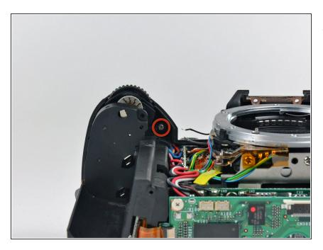
Remove the 4.7 mm Phillips screw from under the top cover near the shutter button.
