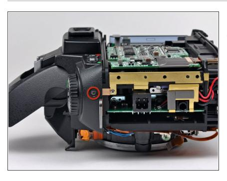
Remove the Phillips screw securing the top cover to the D70 near the mode dial.
