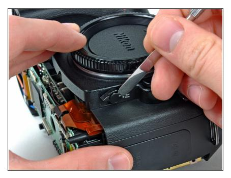
Use the sharp end of a metal spudger or a razor blade to peel the sticker out of the center of the automatic/manual focus switch.
