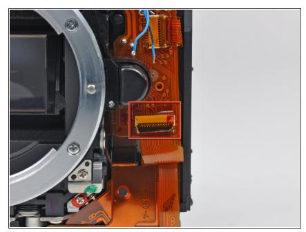
i If present, remove the piece of tape covering the ribbon cable socket (boxed in red).
