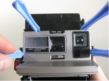
Use several plastic opening tools around the edges of the camera's body to separate it from the plastic frame.
