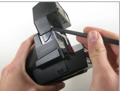
Use a spudger on each side to separate the flash segment from the main body.
