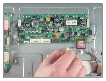
Remove the connector on the bottom right corner by 1st removing tape first and pulling with hand.
