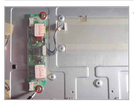
Remove the two screws on the top and bottom of the CCFL inverter with #2 Phillips head screwdriver.
