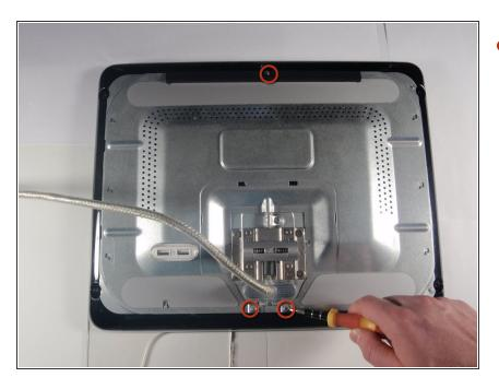
Remove the three screws with #2 phillips head screwdriver.
