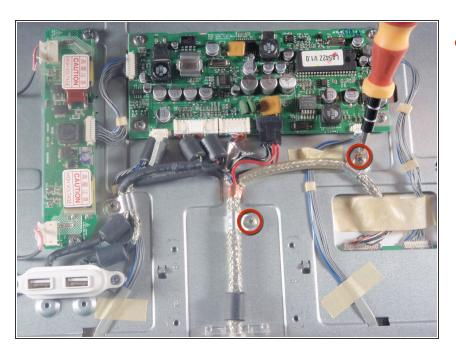
Remove the two philips head holddown screws with the #2 Phillips head screwdriver.
