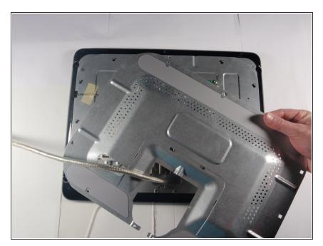
To remove the metal panel, push towards the bottom of the monitor to release its clips and pull the panel away.
