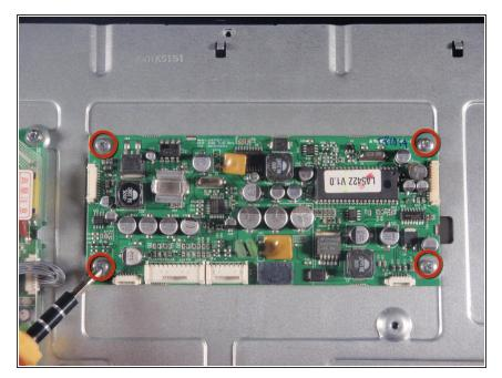
Remove the four screws on each corner of the main board with #2 Phillips head screwdriver.
