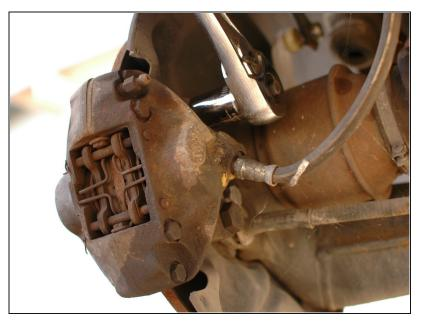
Then tighten the bolts down until they seat against the caliper. Do not tighten them all the way down with the normal ratchet wrench.
