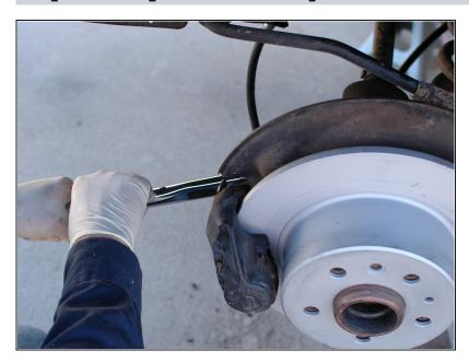
Switch your 19mm socket to a large 1/2 inch drive torque wrench. Torque both of the caliper bolts down to 115 nm/85 lb-ft.
