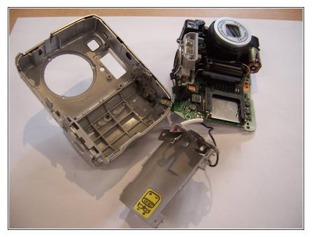
Pull off the battery casing from the inside of the outer front casing. The circuit board, battery casing, and front outer casing will be attached by a connecting strip along with red and black wires.
