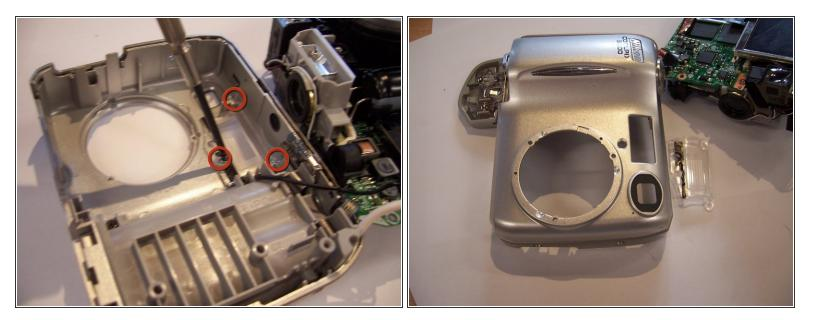
Use a Philips screwdriver to remove the three screws that hold the flash cover to the outer front casing.
