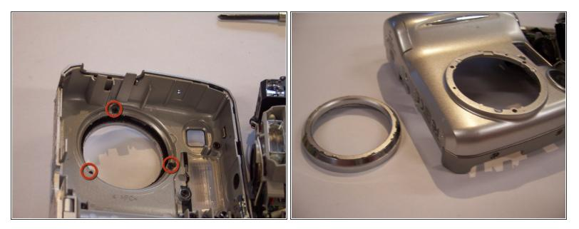
• Use a Phillips screwdriver to unscrew the three screws that connect the outer lens rim to the front casing.
