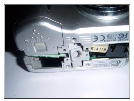
Pry apart the outer casing. A gray plastic threaded piece (used to attach camera to a tripod) will fall out.
