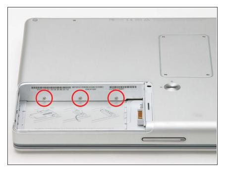
Remove the three 2.5mm Phillips screws from within the battery compartment.
