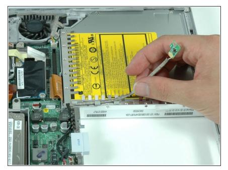
Deroute the cable connecting the hall effect sensor board to the DCto-DC board.
