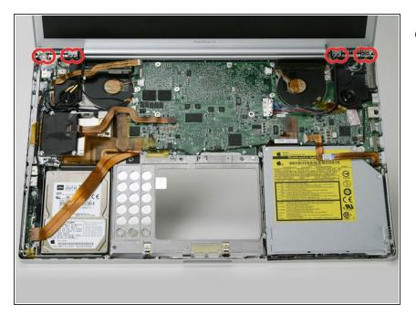
From each complete hinge assembly, remove two Torx T6 screws from the outside of each set, leaving two remaining in the middle of each hinge. On each side, the two screws closer to the edge of the computer are shorter than the two screws closer to the center of the computer. Then remove the two inner screws from each hinge assembly. There are 8 screws total.
