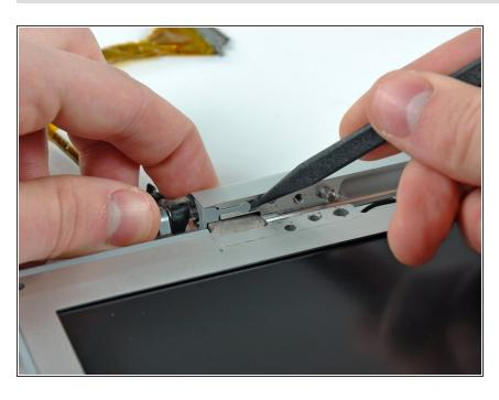
Use the tip of a spudger to remove the plastic end cap from the right side of the clutch hinges.
