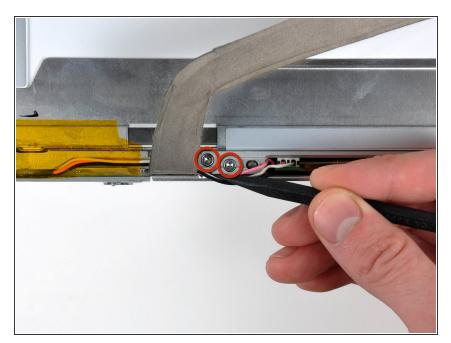
Remove the two 10.3 mm T8 Torx screws securing the left side of the clutch hinges to the front bezel.
