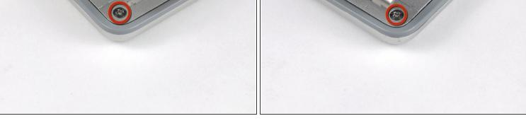
Remove the single Phillips screw from the lower left and right corners of the display.
