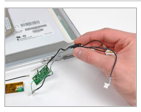
De-route the inverter/antenna cables from the front display bezel.
