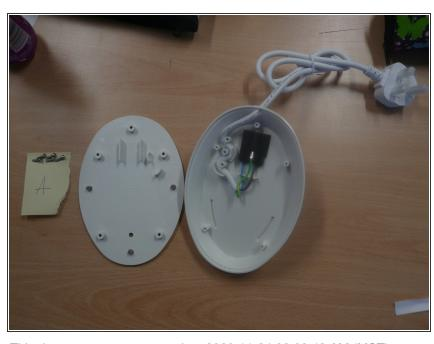
Remove all the screws from the bottom, then gently separate the two halves.
