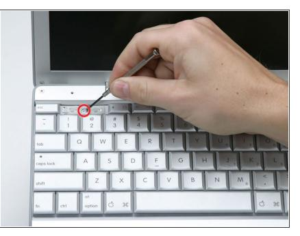
Use your fingernail or a small flathead screwdriver to peel up the gray stickers covering each of the screws.
