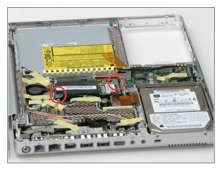
• Remove the two Phillips screws from the corners of the modem.
