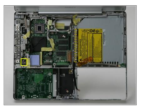
Disconnect the two connectors on the left side of the computer near the ports.
