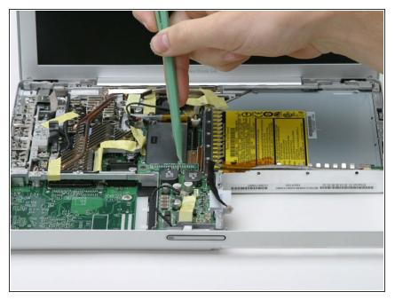
• Lift the end of the DC-to-DC board closest to the display and pull the board out of the computer.
