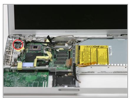
• Remove the single Phillips screw from the RJ-11 board.
