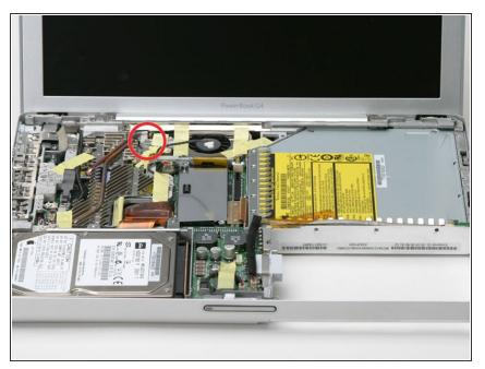
• Remove the single Phillips screw fastening the inverter cable.
