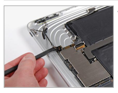
Disconnecting the volume, power, and screen rotation lock buttons connector.
