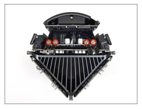
Remove the four 5.5 mm T8 Torx screws securing the power supply assembly to the Mac Pro.
