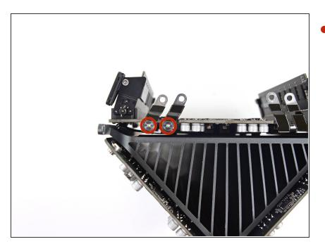
Remove two 5.5 mm T8 Torx screws.
