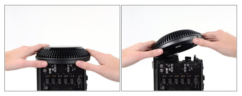
(i) The fan assembly is attached to the rest of the computer by two cables on the IO board side.
