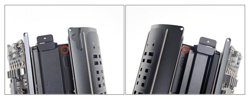
Remove the two 3.6 mm T5 Torx screws from the sides of the power supply cage (one on each side).
