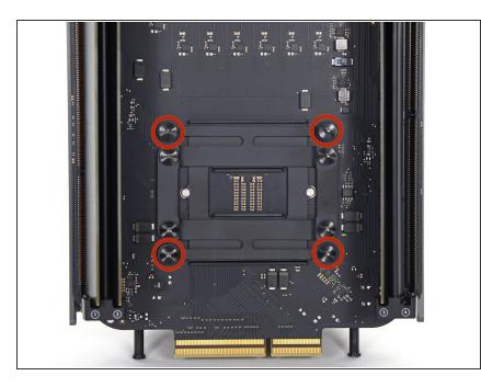
Remove four 12.8 mm T10 Torx screws from the CPU heat sink bracket.
