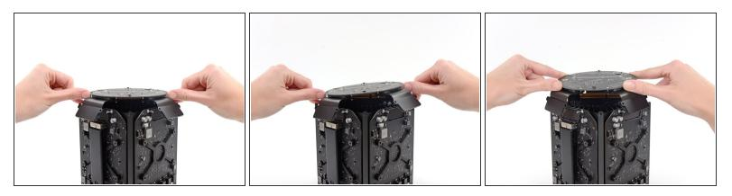
• Gently walk the interconnect board straight up off the logic board's slot connection.
