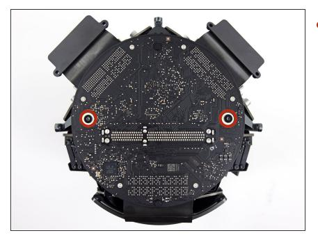
Remove the two 6.0 mm T8 Torx screws securing the interconnect board to the heat sink.
