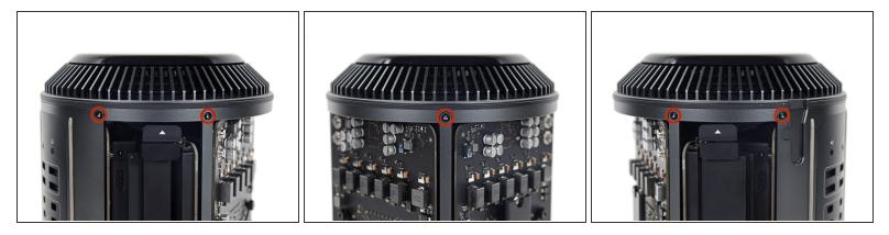
• Remove five 5.1 mm T10 Torx screws from around the outer perimeter of the fan assembly.
