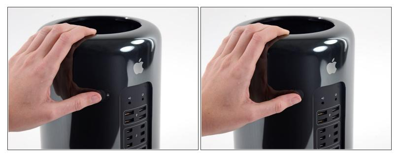
• Slide the lock switch to the right, to the unlocked position.
