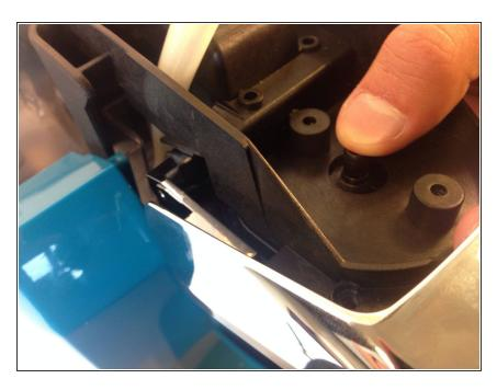
Push down lightly on the nozzle that the hose was attached to. The plastic housing along with the needle should pop off without much force.
