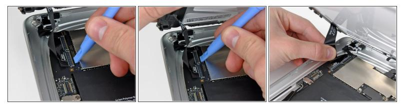
• Use the edge of a plastic opening tool to flip up the retaining flaps holding the digitizer ribbon cables in their sockets on the logic board.
