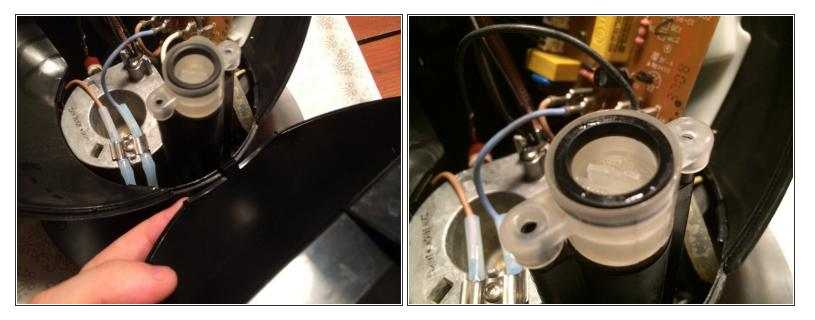
Put it all back together... First the filter, then the rubber ring... You need the smooth side of the ring facing up.
