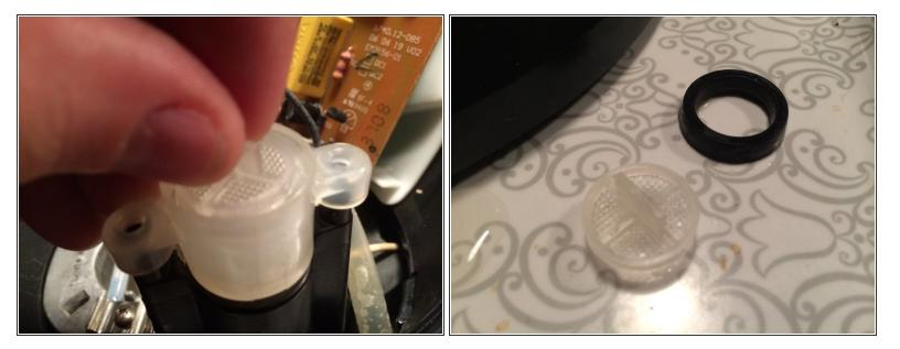
Pull out the rubber seal and the filter.
