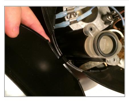
Hook back in the back cover, be careful not to break the clip at the bottom
