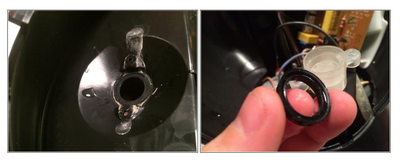
Clean the inside of the cover, the rubber ring, the filter and the holder of the rubber and filter.
