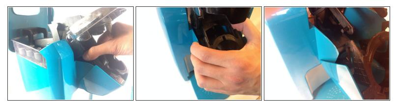
Push in on one of the arms attached to the K-cup holder plastic housing to remove it from its rails. The arms are identical for both sides so once one side is free repeat the process for the second side.
