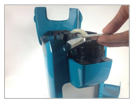
• With the needle removed, open the device by pulling up on the handle.
