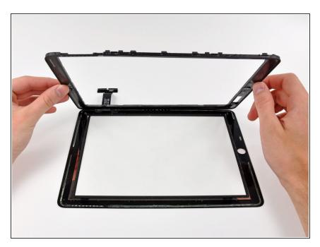
Remove the display frame from the front glass, being careful not to rip the digitizer cable in the process.
