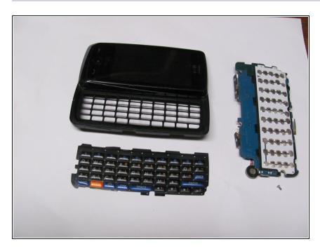
The mother board will fall out of the back along with the silicon keyboard pad.
