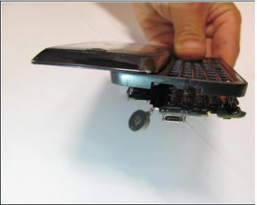
Carefully push the mother board through by pressing into the keyboard.
