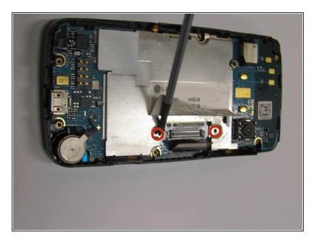
Unscrew two 2mm #00 screws located behind the white serial code sticker.
