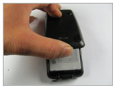
Remove the phone's back cover by placing your thumb the above charging port, located at the bottom of the phone, and sliding the back cover upward.
